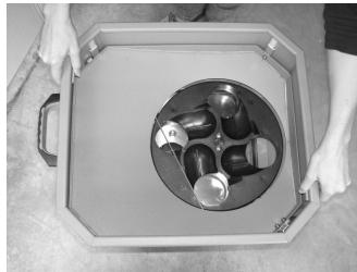
B. Push the hopper down while depressing the hopper release levers.
