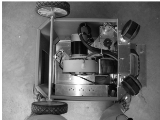
D. In order to get the motor module to go all they way in, you need to point the yellow wheels as shown above and possibly wiggle the wheels small amounts while pushing the motor module down and in.
