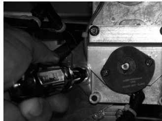
E. Use the (1) nut removed from before and while using the included 7/16 nut-driver, tighten the (1) nut as shown above.
