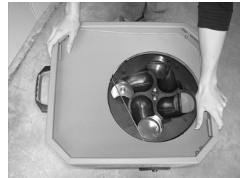
C. Release the hopper release levers.
