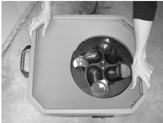
A. Pull up on the hopper release levers.
