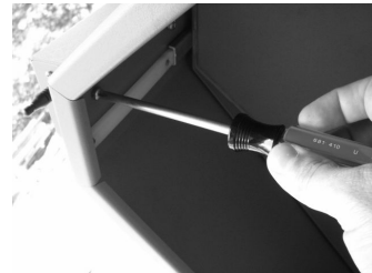
C. Use a #2 Phillips-head screwdriver to tighten the (2) screws and washers.
