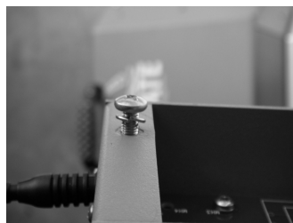
B. Using the #2 Phillips-head screwdriver, completely unscrew the (2) screws and washers.
