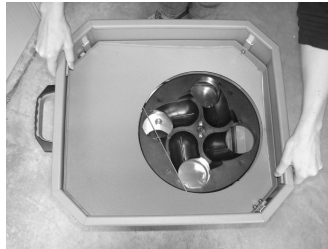
B. Pull the hopper up while depressing the hopper release levers.
